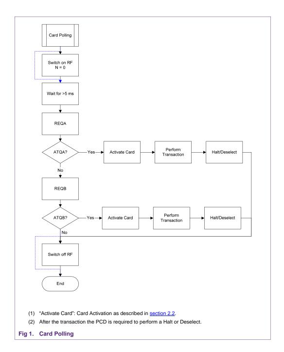
In some applications it might be required to reset the RF regularly, in some others the carrier is switched on only for a short time anyway. In all cases every communication starts with a REQA (or REQB). If an ATQA (or ATQB) is received, the "Activate Card" procedure as described in <a href="section 2.2">section 2.2</a> selects the detected card. If no ATQA (or ATQB) is received, the REQB (or REQA) is used.
